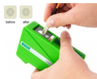
cleaning of fiber optic connectors
